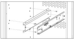
Figure 2. Mounting of side bracket
